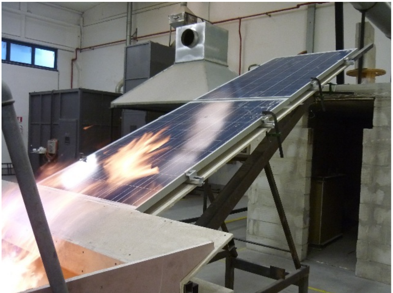
Figure 2 – Spread-of-flame test (LAPI laboratory)
